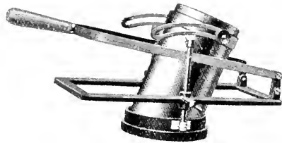
FIG. 69.—Extension tube of a Kidwig compressor to show method of compression. (Siemens.)
